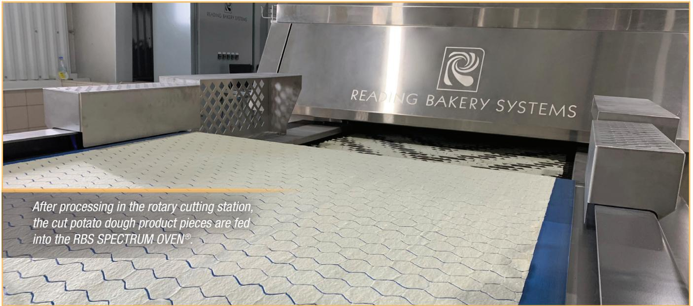
*After processing in the rotary cutting station, the cut potato dough product pieces are fed into the RBS SPECTRUM OVEN®.*
